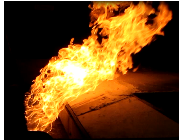
Without 12 mph airflow Diffusion flame
